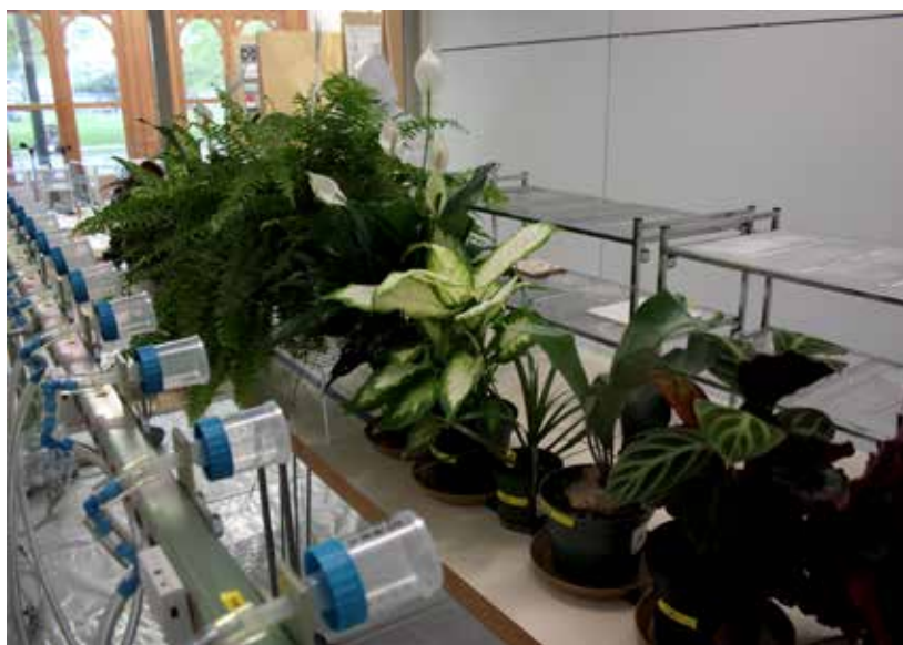
An air vacuum sampling array detects the "microbial clouds" emitted from a cohort of houseplants, here operating during an experiment in a tightly-controlled climate chamber in Portland, OR. The experiments are being conducted by the Sloan-supported Biology of the Built Environment (BioBE) Center at the University of Oregon. (PHOTO COURTESY OF BIOBE CENTER.)
